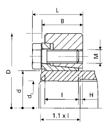
B mm = 29.0 d H8 mm = 55 D mm = 100.0 ds mm = 42 F kN torque = 62 H = 3.0
